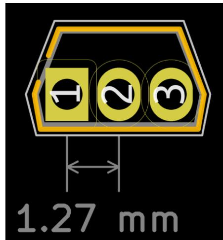
TO-92S footprint with standard lead spacing.
