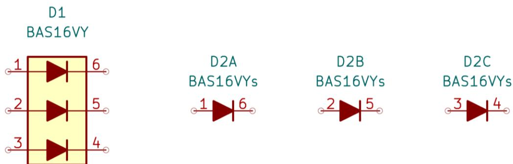
**Figure 2.4** Triple diode symbol that has two variants:
