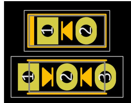
*Vertical rectangular 5x2mm LED (top) and a common-cathode 5x2mm LED (bottom)*
