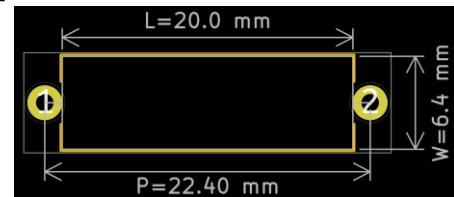
*Power resistor footprint with relevant dimensions indicated.*
